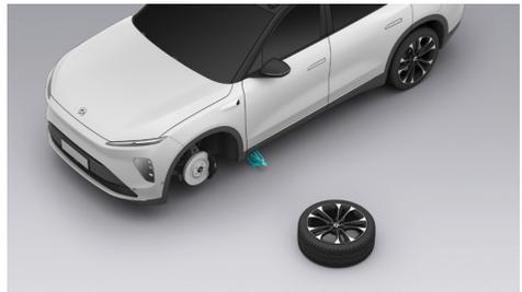
7. Remove the wheel bolts and replace the tire. When installing the wheel, make sure the bolts are aligned with the mounting holes, and that the metal side of the wheel is in proper contact with the mounting surface.
