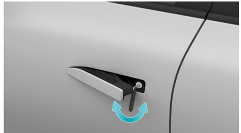
4. To lock the vehicle, you can use the mechanical key to turn the groove in the keyhole on the side of the door to a vertical position. Once the door is closed, it will be locked.
