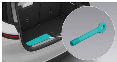
2. Press the lower end of the front towing flap of the vehicle to open it (1 in the figure), insert the hitch into the hole and rotate until the hitch is firmly seated (2 in the figure). The rear hitch (if present) is installed in the same way as the front hitch.
