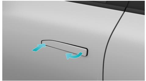
3. Hold the unfolded outer door handle with one hand while inserting the physical emergency key into the keyhole in the outer door handle with the other hand, and turn the key clockwise to unlock the driver's door.
