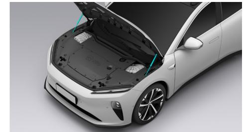
3. Disconnect the emergency high voltage cutoff plug to cut off the high voltage circuit. Remove the plug and stow it properly.
